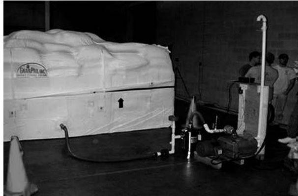
FIGURE 8.8 A V-HF Cocoon holding cocoa beans in bags, under a pressure of 50 mm Hg connected to the vacuum pump in a trial site in Boston, MA.
